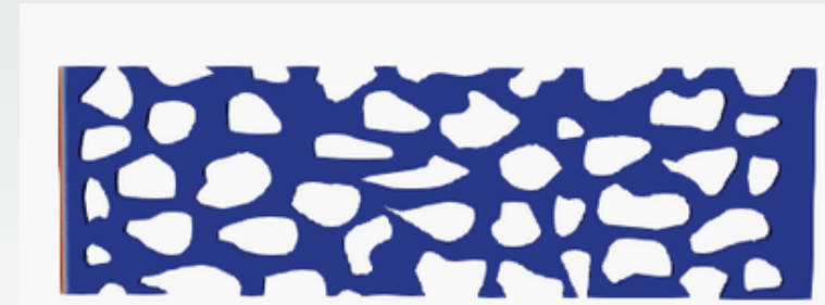
Evolution of CO 2 /brine phase distribution during drainage in a 2D porous medium.
