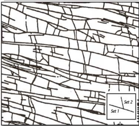
Typical Reservoir Fracture Pattern, MWX Site.
