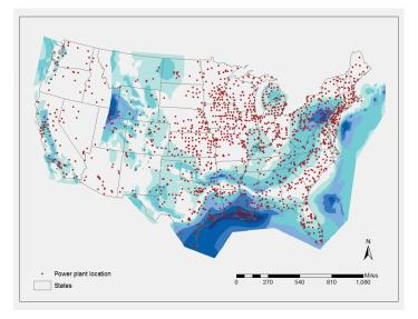
Sources and sinks: Red dots show sources of  $CO_2$ . Colored zones show places in the U.S. with geological formations appropriate for CCS. Texas, in particular, is well suited for injecting  $CO_2$  into deep underground containment zones.
