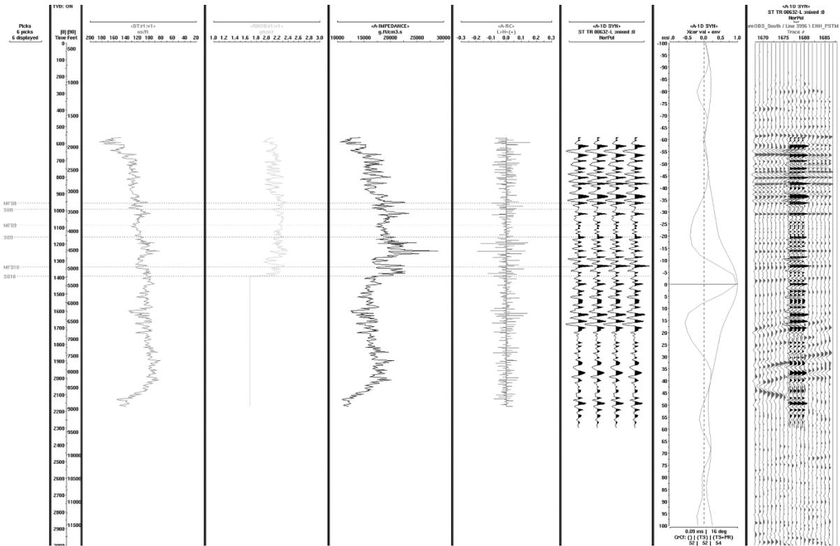
Figure 2.1.1.2.7 – Synthetic seismogram for time/depth correlation.
