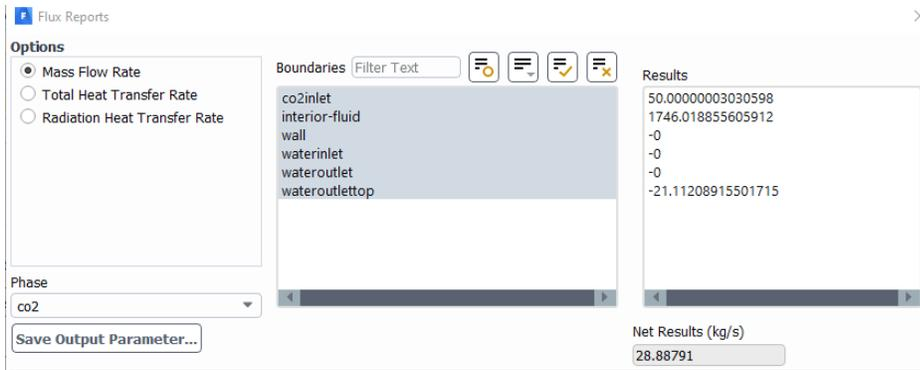
Figure 4.1.5.2 CO<sub>2</sub> Mass Balance
