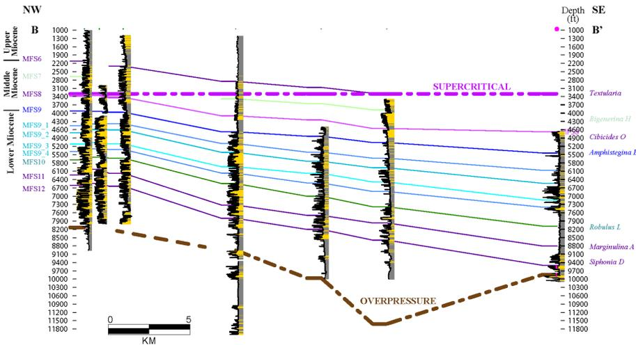
Figure 2.1.1.2.2 – Dip-oriented structural cross-section, offshore Texas coast (BB' in Figure 2.1.1).
