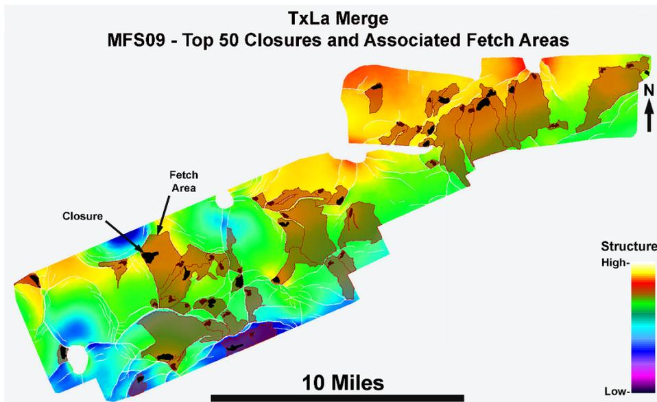
Figure 2.1.1.1.2 – TexLa Merge 3D - MFS09 structure map with top 50 closures and associated fetch areas.
