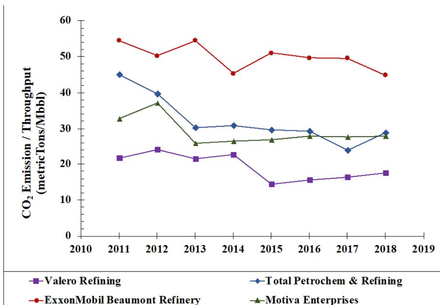
Figure 5.5. CO<sub>2</sub> Emissions/Capacity (metric Tons/Mbbl)
