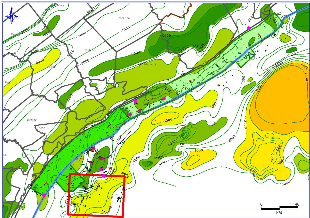
Figure 2.1.1.2.4– Map of the study area from Corpus Christi to Galveston Counties showing the 3D seismic surveys (highlighted in green and red). The map contours are from (Burke et al., 2012) top of overpressure grid. The state - federal waters boundary is demarcated by the blue line subparallel to the coast. The top of the overpressure is very shallow (4000-5000 ft) in the federal waters immediately southeast of the state waters offshore Matagorda and Corpus Christi Bays.
