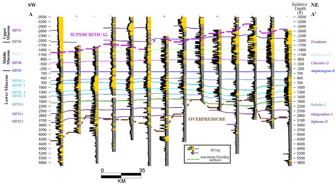
Figure 2.1.1.2.1 – Strike-oriented stratigraphic cross-section, offshore Texas coast between Galveston and Matagorda Bay (AA' in Figure 2.1.1). The cross-section is flattened on MFS9 (*Amphistegina B*).
