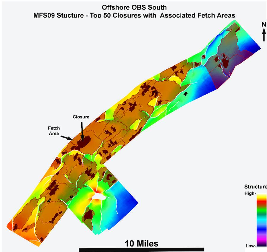
Figure 2.1.1.2.6. Offshore OBS South 3D - MFS09 structure map with top 50 closures and associated fetch areas.
