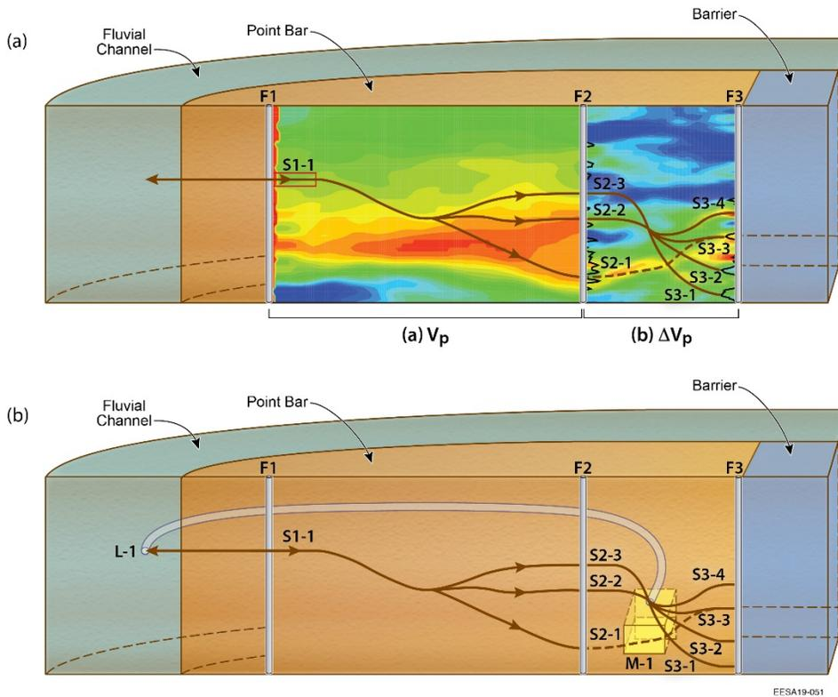
Figure 3.1.4.1 Diagram of the fluvial-channel-point-bar system at the DAS site with (a) small-scale flow channels imaged during the early  $\text{CO}_2$ -plume development and (b) the network of large-, intermediate-, and small-scale flow channels imaged during the late-time plume development
