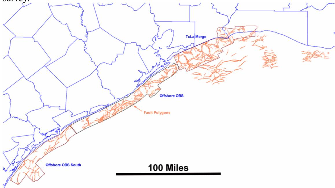
Figure 2.1.5 – Regionally interpreted MFS09 fault polygons, including the Offshore OBS South 3D survey. There are 709 fault polygons in this image.
