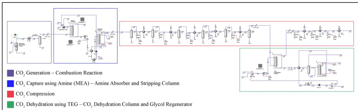
Figure 5.2.1. Process diagram for the separation, compression, and dehydration of CO<sub>2</sub> from flue stack gases
