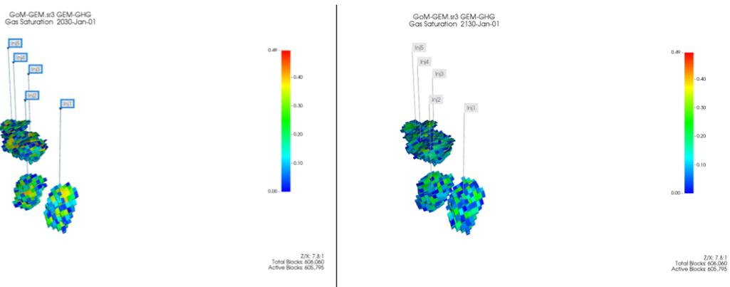
Figure 5. CO<sub>2</sub> plume at the end of injection (left) and post-injection (b) periods for scenario 5.
