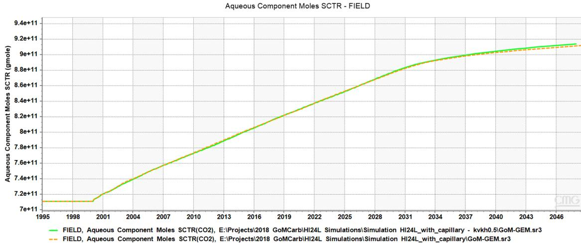
Figure 4. Time evolution of CO<sub>2</sub> dissolved into the brine for scenarios 1 and 4. Higher kv/kh ratio has slightly increased the amount of CO<sub>2</sub> dissolution into the brine.
