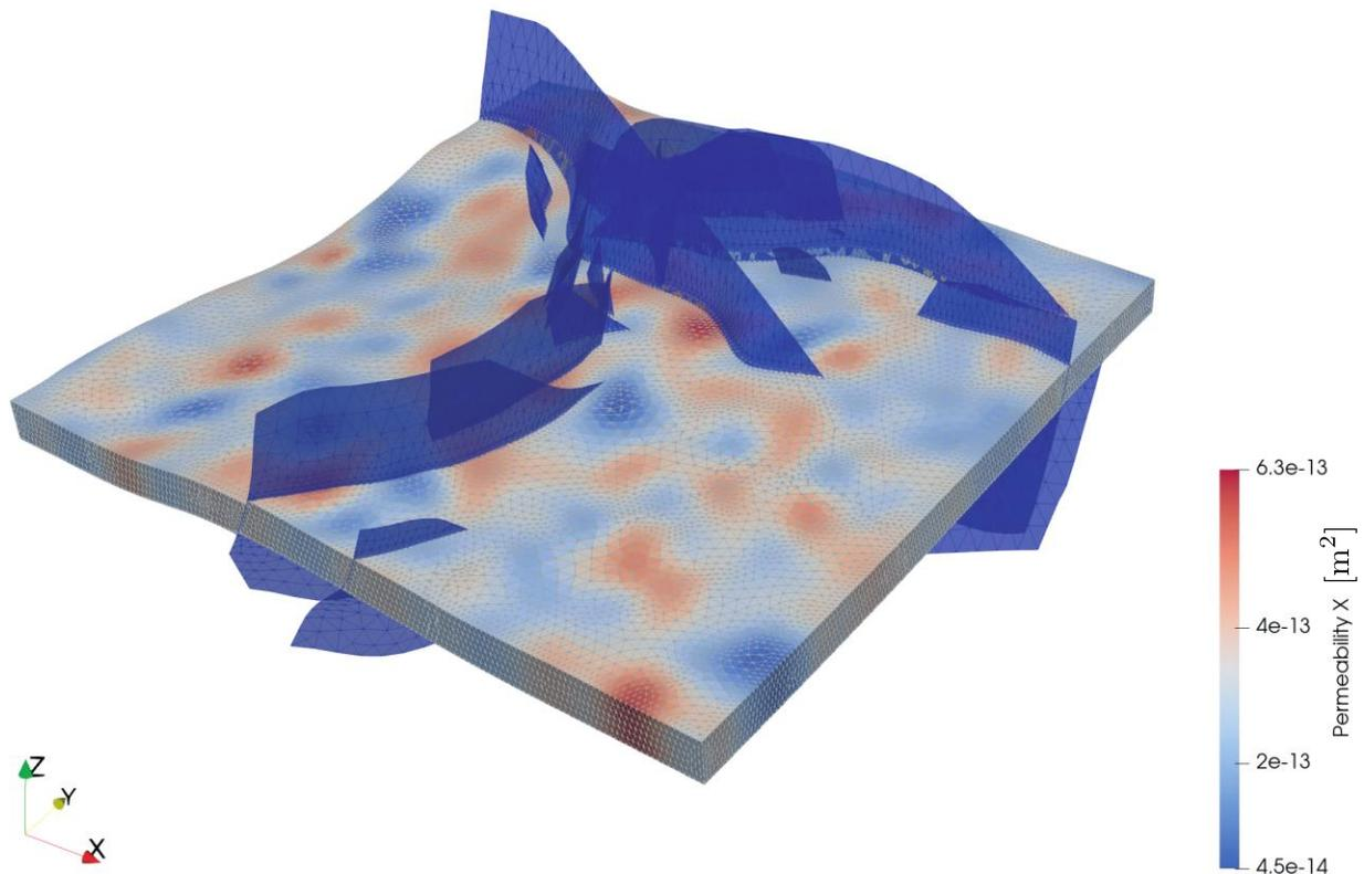
Figure 3.2.1 Horizontal permeability distribution in the reservoir, statistically generated. The faults cutting the domain are illustrated in blue.
