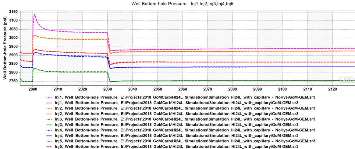
Figure 6. comparison of BHP values in scenario #1 vs. scenario #5 for all 5 injection wells.
