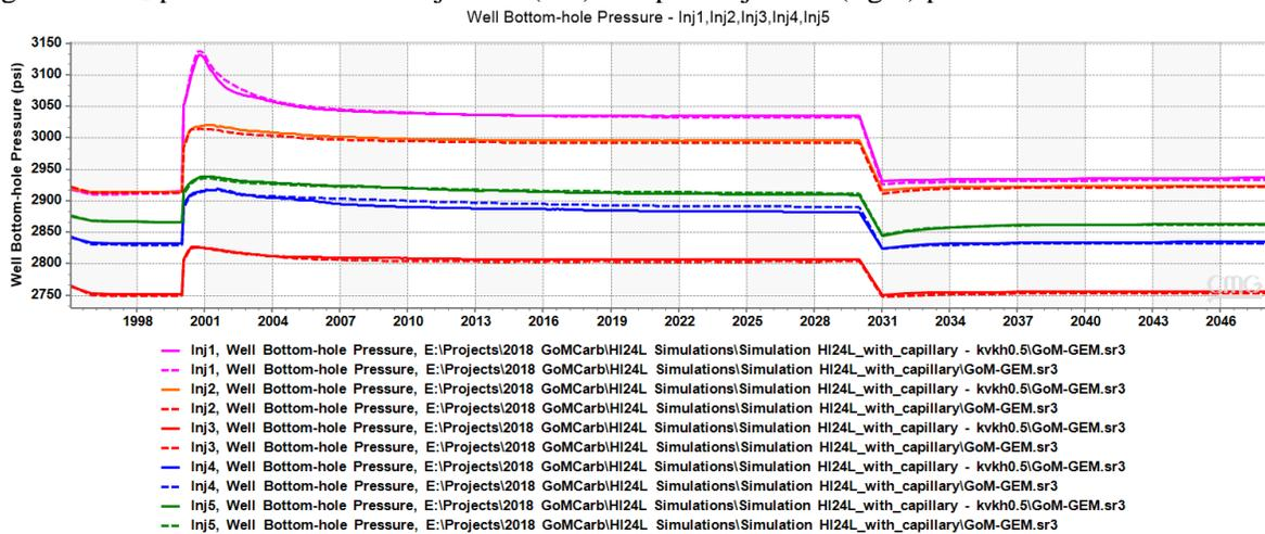
Figure 3 comparison of BHP values in scenario #1 vs. scenario #4 for all 5 injection wells.
