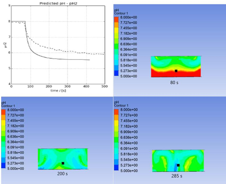
Figure 4.1.5.1 Measured vs. predicted pH in Cussler et al. 's work (Top Left, [2]) and pH profiles at various time intervals from CFD Simulations in this study (Top Right and Bottom figures).
