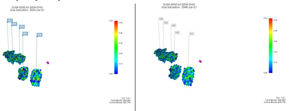
Figure 2. CO<sub>2</sub> plume at the end of injection (left) and post-injection (right) periods for scenario 4.
