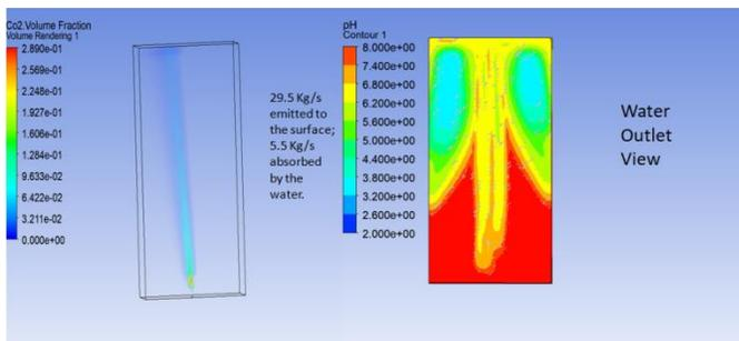
Figure 4.1.5.3 Simulation Results CO<sub>2</sub> Plume (L) and pH Variation (R)
