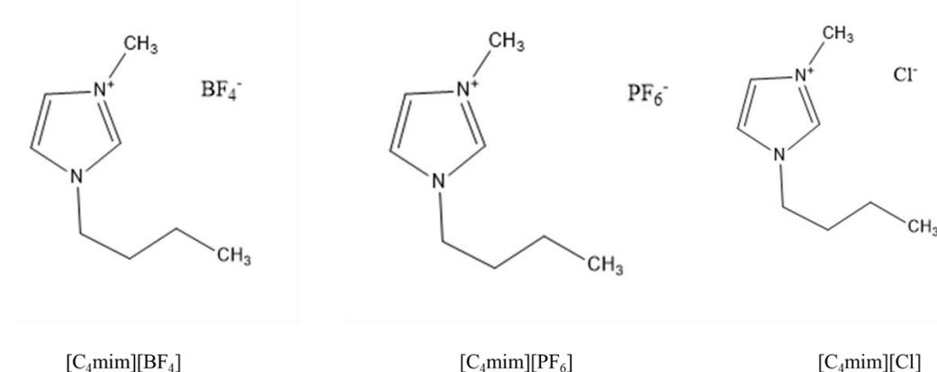
Figure 5.2.2. Ionic Liquids that have been identified for CO<sub>2</sub> solubility where the cations contain the organic constituent, and the inorganic constituent contains the delocalized charge. [C<sub>4</sub>mim] = 1-butyl-3-methylimidazolium.
