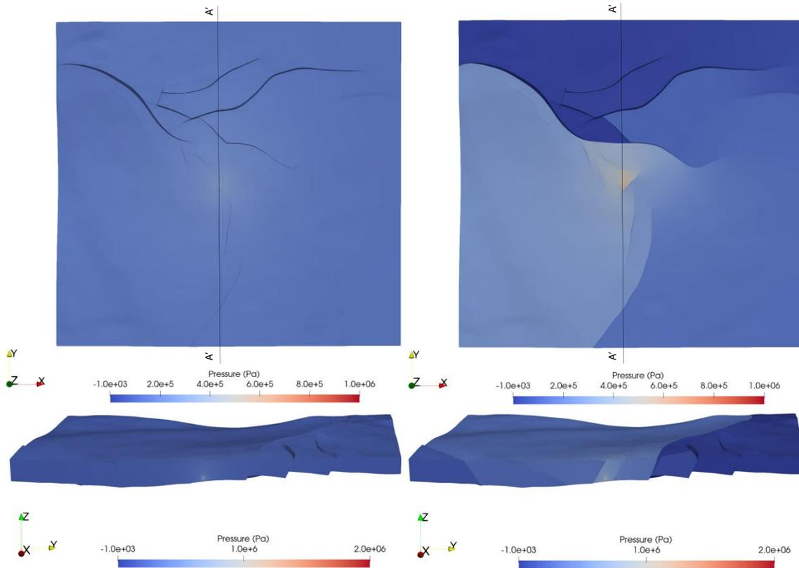
Figure 3.2.2 Simulation results for the base case scenario. Excess pore pressure after 3 years of injection at a rate of 1 Mt/yr for two cases: permeable faults (left) and impermeable faults (right) for top and lateral views of the reservoir.
