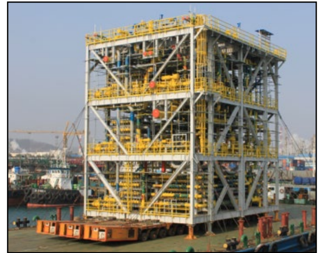
CO 2 unit using the UOP spiral wound membrane.
