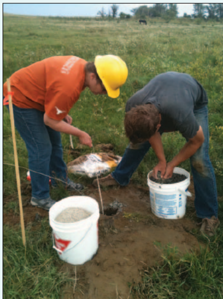
Hilary Olson and Thomas Ogilvie prepare a soil gas sampling well to investigate claims of carbon dioxide leakage beneath a farm in Saskatchewan, Canada.
