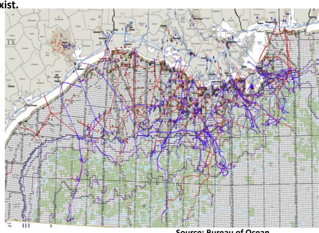
Oil Pipelines in Blue Gas Pipelines in Red
