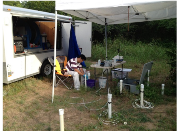
Monitoring a push-pull test at the Brackenridge Field Laboratory
